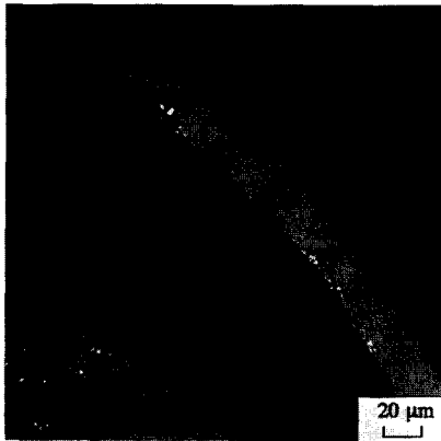
Fig. 2. Typical example of corrosion of the SiC layer by the fission product palladium in a Triso-coated UO_2 particle irradiated to 3.8% FIMA at 1480°C.
